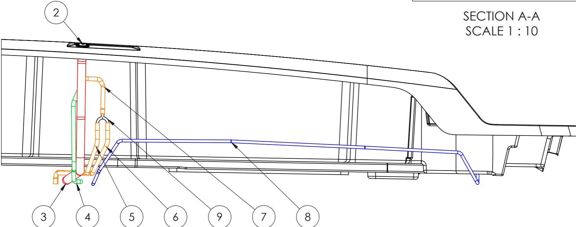
Fuel hose supply route fixed onto the deck on the PS
