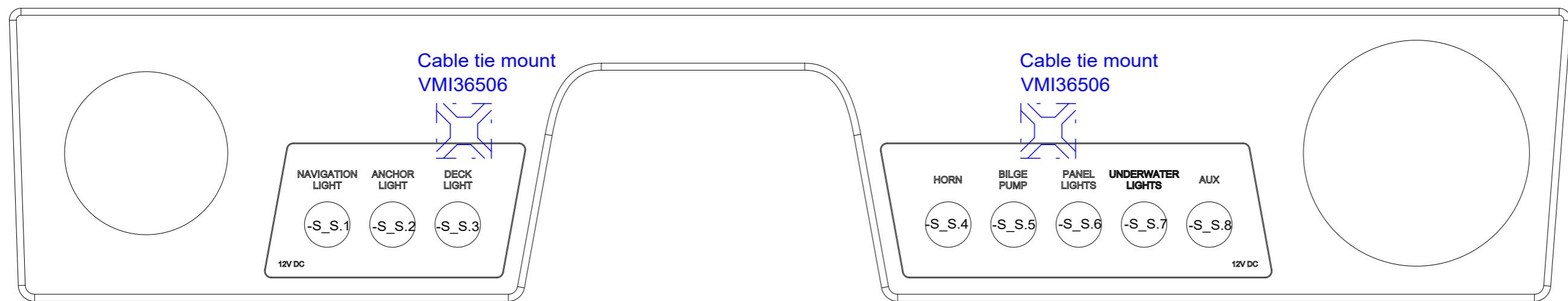
1. Install the Cable Tie Mounts on the back of the panel, using double-sided tape attached. As in the pictures. (Clean the panel surface first.)
